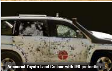
Armoured Toyota Land Cruiser with IED protection
