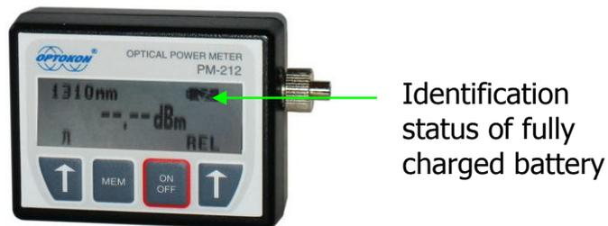
Figure 2: Status of fully charged battery
