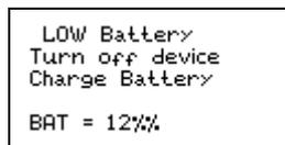
**Fig. 3:** Device display at the low battery charge level.
