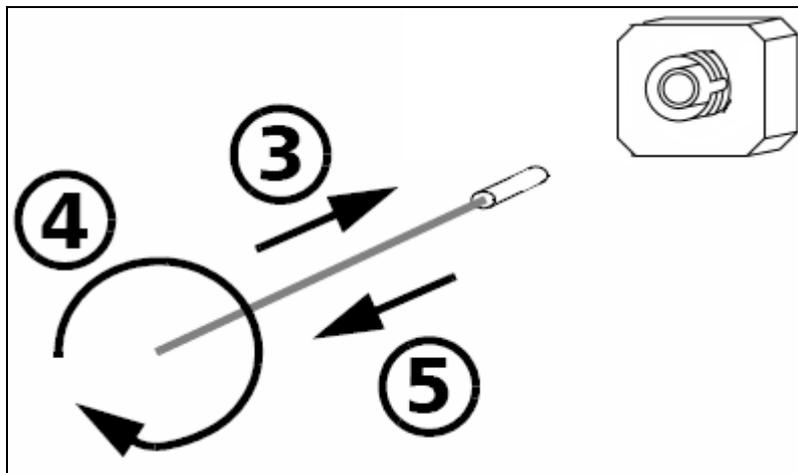
Fig. 28: Connector cleaning.
