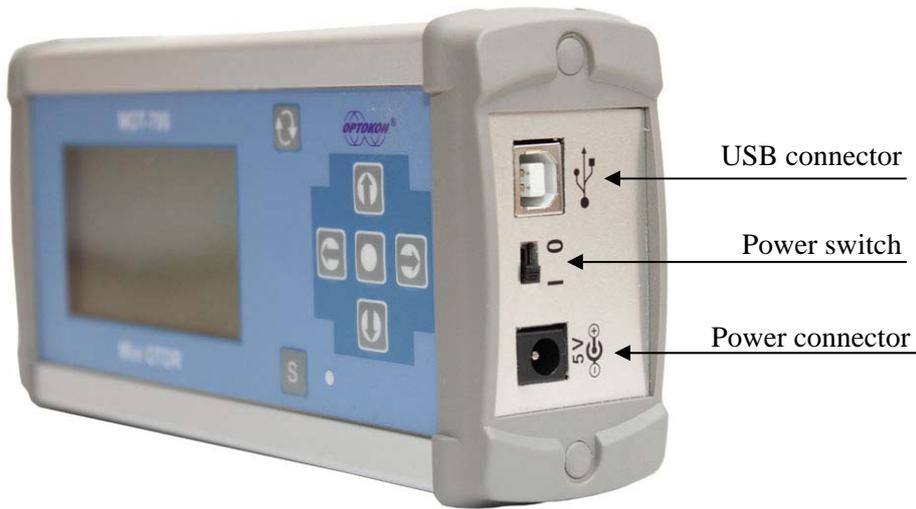
**Fig. 2:** Device appearance (side view).
